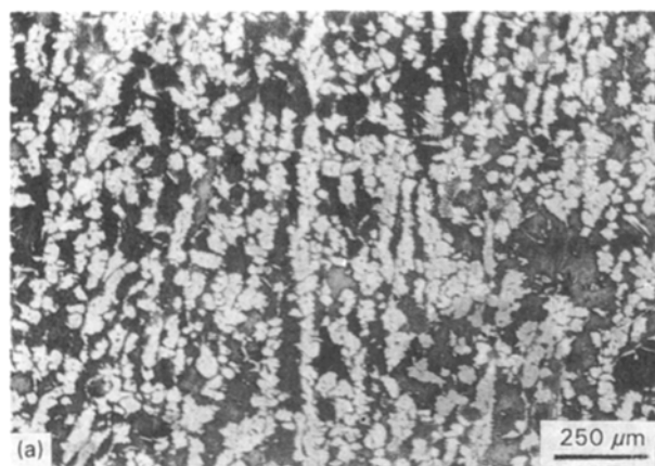
Figure 4 (a, b) Microstructure of \alpha - \beta nickel silver specimen deformed at 850^{\circ}\text{C} and 0.01\text{ s}^{-1} showing globularized \alpha phase, at low and high magnification, respectively.
